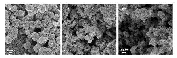
Figure 3. SEM images: (a) ZnO, (b) ZnO:Cu 5% and (c) ZnO:Co 5% thin films.
