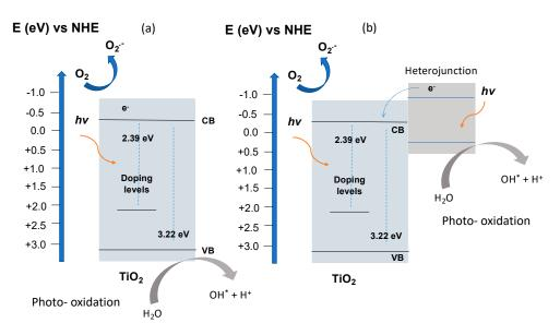
**Scheme 1.** Hypothetical scheme of energetic levels for metal-doped ZnO thin films: (a) Metal doping process. (b) Metal doping process and the generation of a heterojunction [64,70,71]. After charge pairs generation, the ROS can be yielded on the catalyst surface and MB degradation starts.
