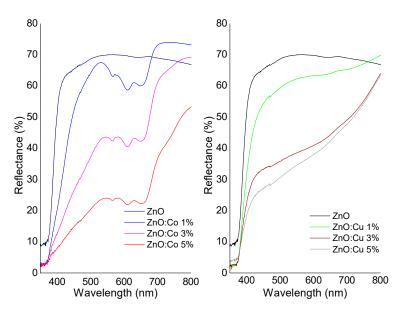
Figure 4. Reflectance diffuse spectra for both catalysts.
