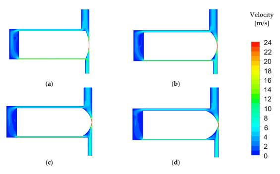
Figure 13. Flow gas velocity through compression ring, (a) profile 1, (b) profile 2, (c) profile 3, and (d) profile 4.
