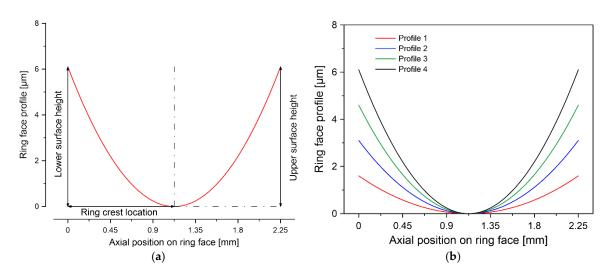
Figure 2. Compression Ring Geometric Profiles. (a) dimensions and (b) geometric profiles.
