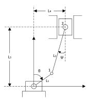
Figure 5. Piston kinematic model.
