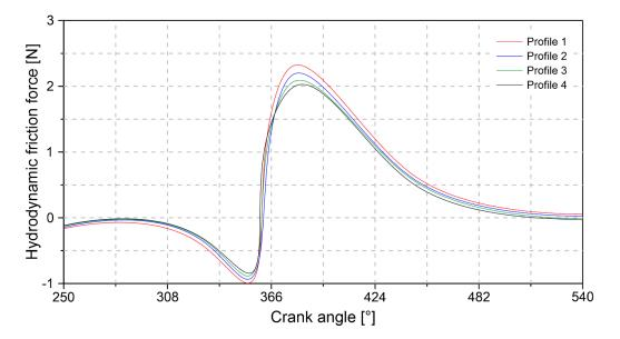
Figure 14. Hydrodynamic friction force.
