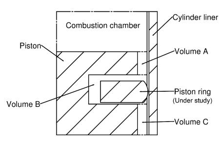
Figure 7. Control volumes for the exhaust flow model (First ring).
