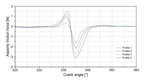
Figure 16. Asperity friction force.
