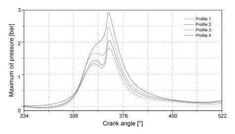
Figure 18. Maximum oil pressure inside of the compression ring.
