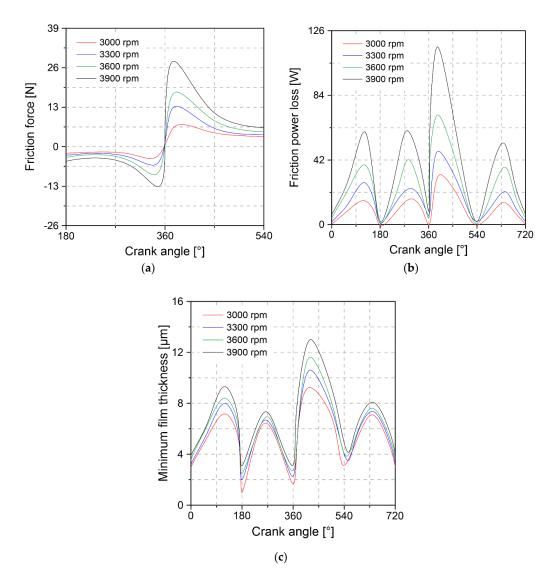
Figure 20. (a) Friction force, (b) friction power loss, and (c) minimum film thickness for a load of 6 Nm.
