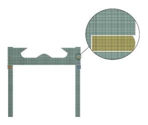
Figure 3. Meshing used for simulation.
