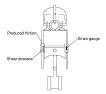
Figure 10. Strain gauge sensor location.
