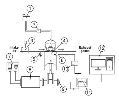
**Figure 4.** Diesel engine test bench. 1. Fuel tank, 2. Fuel control valve, 3. Air flow indicator, 4. Engine diesel, 5. Thermocouple, 6. In-cylinder pressure transductor, 7. Dynamometer controller, 8. Dynamometer, 9. Crank angle encoder, 10. Charge amplifier, 11. Combustion data acquisition system, 12. Computer.
