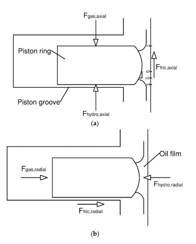
Figure 6. (a) Axial forces and (b) radial forces on the piston compression ring.
