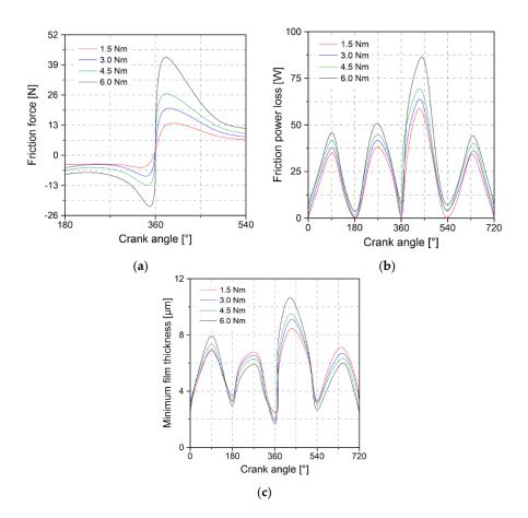
**Figure 22.** (a) Friction force, (b) Friction power loss, and (c) Minimum film thickness for an engine speed of 3500 rpm.
