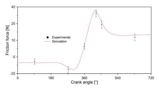
Figure 12. Comparison between the friction force obtained experimentally vs. CFD simulation.
