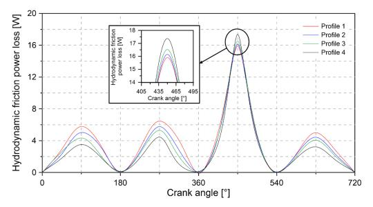
Figure 15. Hydrodynamic power losses for each geometric profile of the compression ring.
