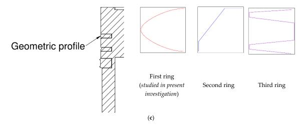
Figure 1. Geometry for the 2D-CFD model, (a) piston, (b) piston cross-section, and (c) rings profile.
