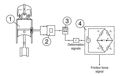
**Figure 11.** Measurement process of the friction force signal. 1. Engine, 2. Signal control board, 3. Data card analysis, 4. Calibration system.
