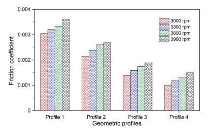
Figure 21. Friction coefficient between compression ring and cylinder liner.
