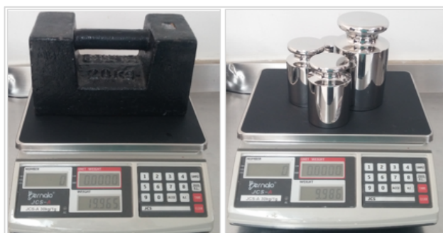
Fig. 1. Bernalo Non-Automatic Weighing Instrument (Capacity: 30.000 kg; Resolution: 0.001 kg)
