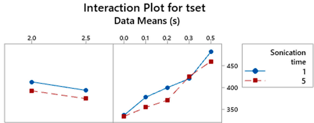
Figure 5. Interaction plot between the effect sonication time vs. BPO/solid ratio and sonication time vs. GO/liquid ratio for the variable t_{set} .
