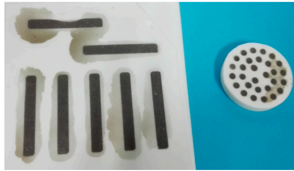
Figure 2. Molds with bending and compression specimens.
